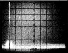
Fig 5—Kenwood TS-690S worst-case 50-MHz spectral display. Horizontal divisions are 10 MHz; vertical divisions are 10 dB. Output power is approximately 38 W at 50.1 MHz. All harmonics and spurious emissions are at least 62 dB below peak fundamental output. The TS-690S complies with current FCC specifications for spectral purity for equipment in this power-output class and frequency range.
